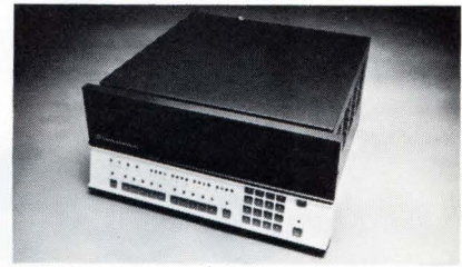
Fig. 2—Add a power supply, a control console with a hexidecimal keyboard and a cabinet to the Naked Mini/LSI and you have an Alpha/LSI.
