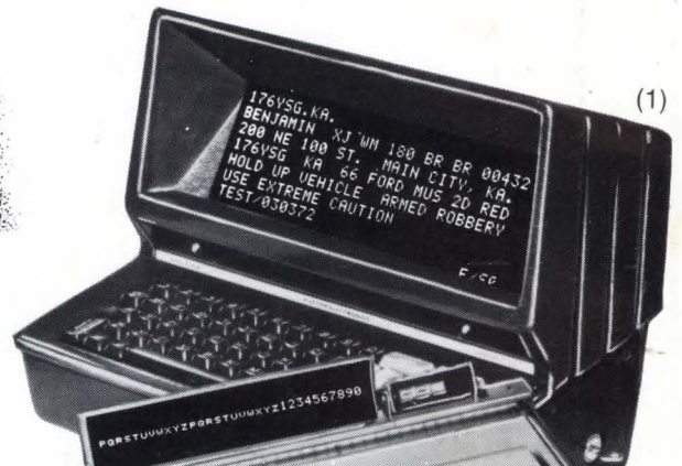
32/37, 80 Character Position Panel, 5 x 7 Dot Matrix, Characters 0.2" High. Alphanumeric panel with 64-character format.
